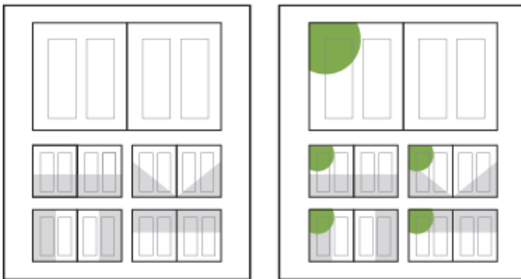
Original parent and child masters (left); when the parent master is modified, the child masters are automatically updated (right)
