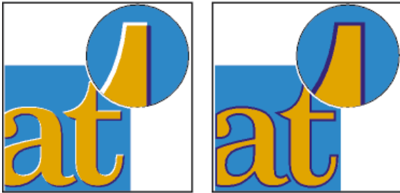
Misregistration with no trap (left) and with trap (right)
