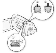
3 Press PHOTO fully. The ACCESS indicator will flash as the photo is being recorded.
